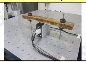
Mechanical Shock Test: -Y axis
