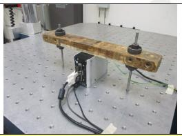
Mechanical Shock Test: +Y axis
